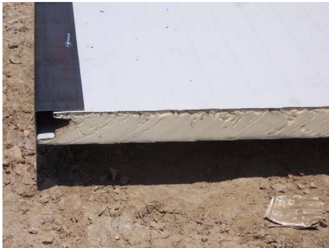
Absorption material for the development of the movable noise barriers at Sperhios river bridge area.
