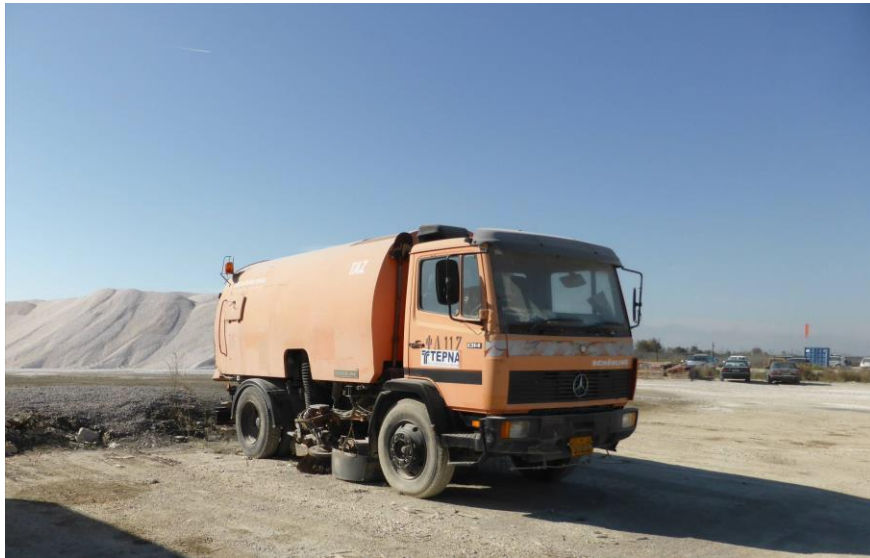
Cleaning vehicle. It is used for the cleaning of paved access roads
