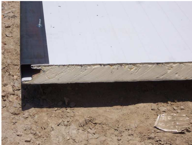
Photo 2. Absorption material for the development of the movable noise barriers at Sperhios river bridge area.
